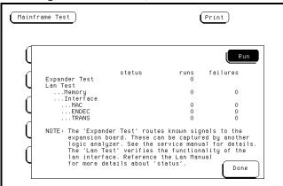
If an HP 16501A expansion frame is not connected, then expect a "No Expander Card Present" message to appear when you run the Option Board Test. Refer to the HP 16500B Service Guide formore information about the expansion frame.
